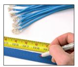
Measure the sleeving to length. Keep the sleeving relaxed and don't pull it as you measure. The most accurate method is to measure the sleeving on the actual application. There will be some foreshortening of the sleeving as it expands over large bundles or connectors. Mark the cut line with a pen or marker.
