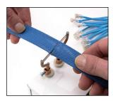
When the knife is hot, slide the sleeving over the cutting blade. Practice on a piece of scrap to get a feel for the procedure. Always cut in a well ventilated area and avoid inhaling the fumes. Both the blade and the cut ends will be HOT. Be careful.
