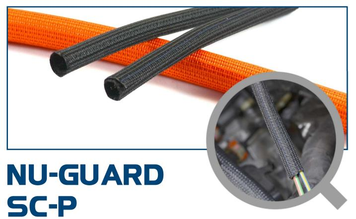
The flat-knit construction of the NU-GUARD SC-P is made of PET monofilament and textured multifilament combination; which gives a lightweight, rugged but yet smooth texture and appearance.
