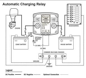
**Note:** Because the ATD is single sensing, the battery connected to the charging source must be attached to the stud labeled "BATT". Reversal of the starting and house batteries will create undesirable results.
