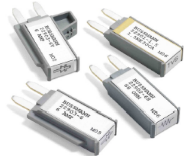
Clockwise from top right: Transorb, Resistor, Diode, and Diode with extended 'wing' key option.
