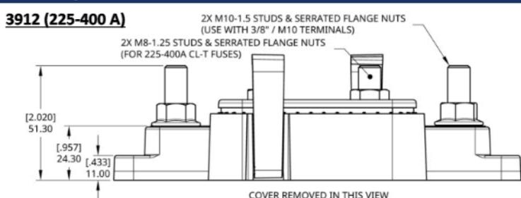
2X M10-1.5 STUDS & SERRATED FLANGE NUTS
