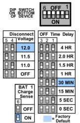
**DS1-DS3** sets delay between Off Trigger and Relay OFF. 0 SEC is for install testing or pure relay functionality without time delay
