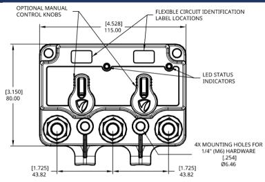
CONTROL CABLES LENGTH 12.0" (304.80). TERMINATION OPTIONS INCLUDE FLYING WIRE LEADS, (2) DEUTSCH STYLE DT/AT SEALED CONNECTOR
