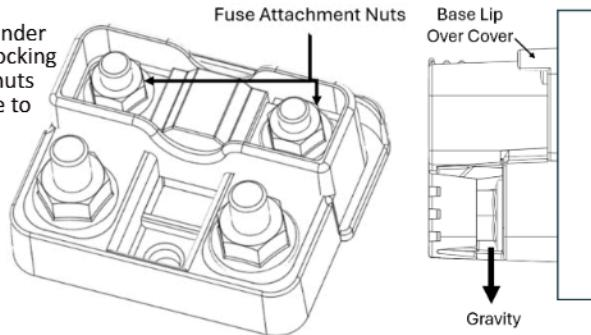
(5) Assemble cover to base and ensure cover latch snaps into place and cover is not able to be removed without depressing the latch release tab.
