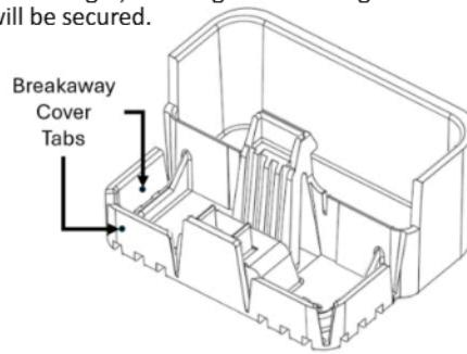
(4) Install fuse under cover with self-locking serrated flange nuts provided. Torque to recommended specifications.
