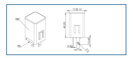
UP TO 14LAMPS INPUT LEAD MUST BE FUSED
