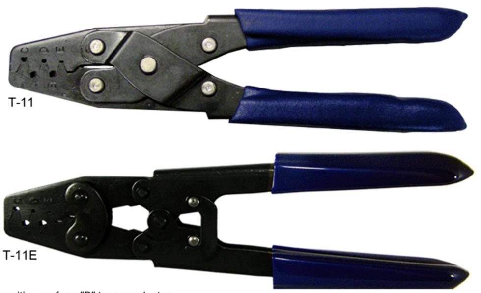
Five cavities perform "B" type conductor and insulation crimps. Conductor maximum crimp range is 22-12 AWG. Insulation maximum crimp range is 24-14 AWG. The T-11 uses the same five crimp cavities as the professional Delphi/Packard 12085271 tool, but is built on a less expensive, non-ratchet frame. (For an exact equivalent to the 12085271, use our T-16 procrimper.) The T-11 is our most popular crimping tool.
