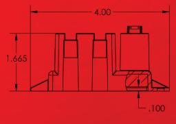
Mounting torque: 35 in-lbs max with M4 or #10 fastener, flat washer and lock washer
