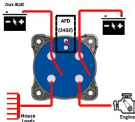
2 Position On/Off Selector **Controls Two Independent** Circuits.
